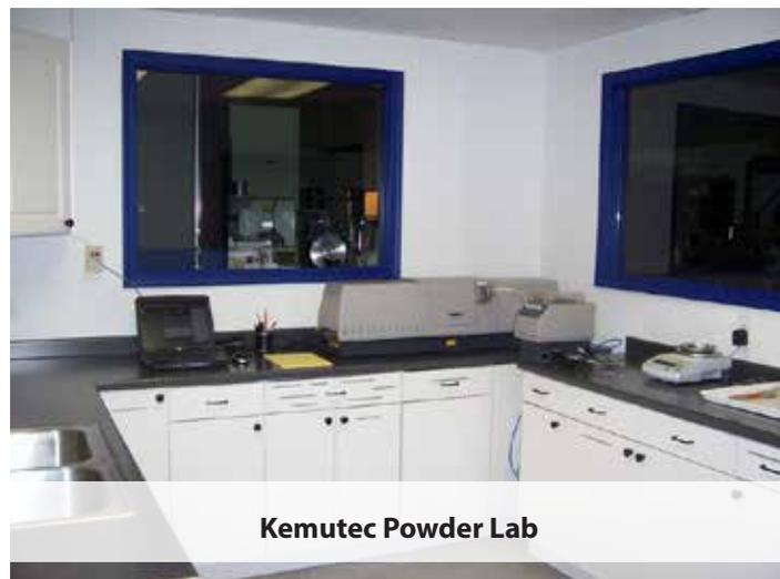
Supporting the testing services, Kemutec has a laser particle size analyzer to facilitate accurate size determination of both the feed and processed test materials.
