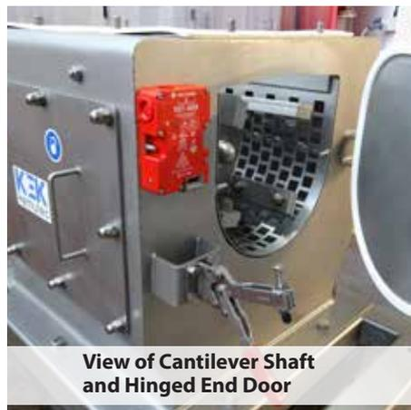
View of Cantilever Shaft and Hinged End Door
